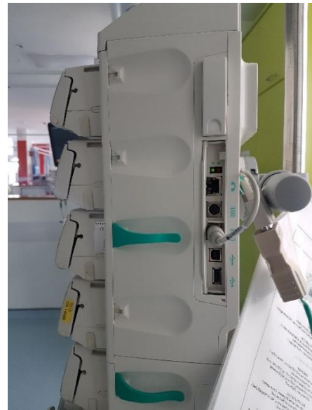
Figure 4-1 Data Capture server in situ & Fig 4-1.2 SIP rack with an RS232 connection situated in PICU, OLCHC
