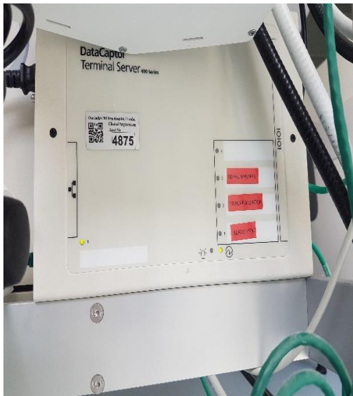
Figure 4-1 Data Capture server in situ & Fig 4-1.2 SIP rack with an RS232 connection situated in PICU, OLCHC
