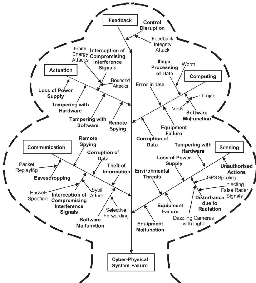
Figure 6: Tree diagram of cyber threats and attacks on a Cyber-Physical System(CPS) [14]
