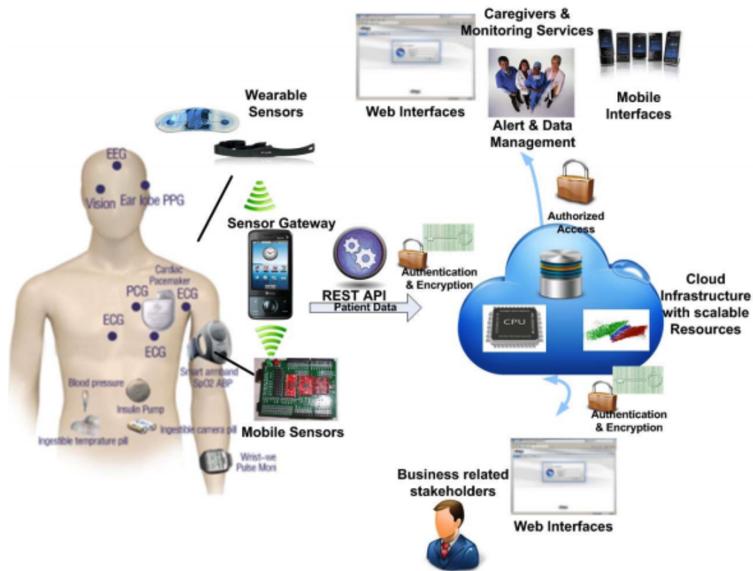
Figure 1.5: An example of a potential architecture for a smart care facility [13]
