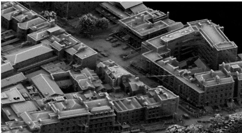
Figure 3.1: An example of high-density LiDAR data in the city of Dublin, Ireland.
