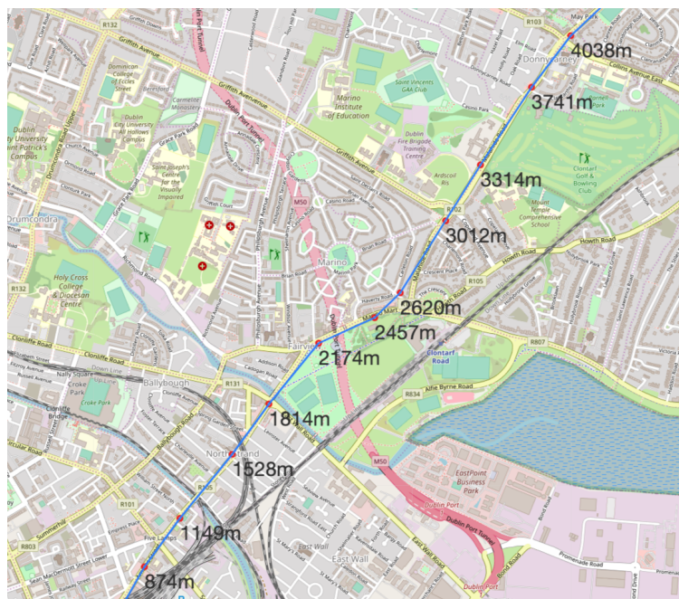
Figure 4.5: The cumulative distances of nodes along a GPS trace of the 27B bus.
