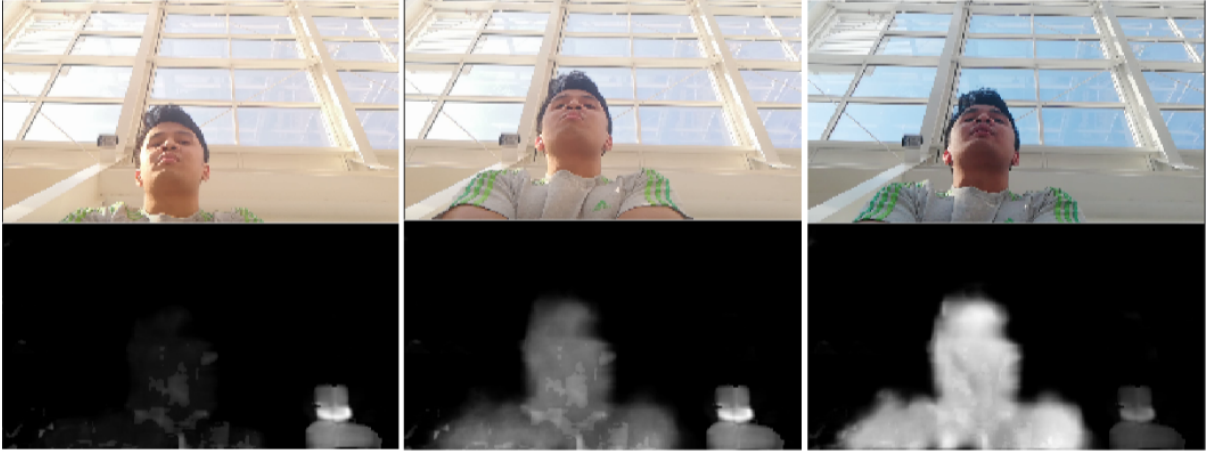
Figure 3.6: The weighted mask after several seconds of CPR time. Note the increasing weight in the region of the user and diminishment of the non-moving area on the bottom-right.
