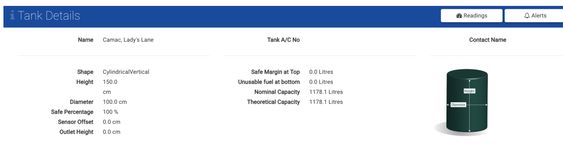
Figure 5.23: VT sensor configurations as displayed on dashboard
