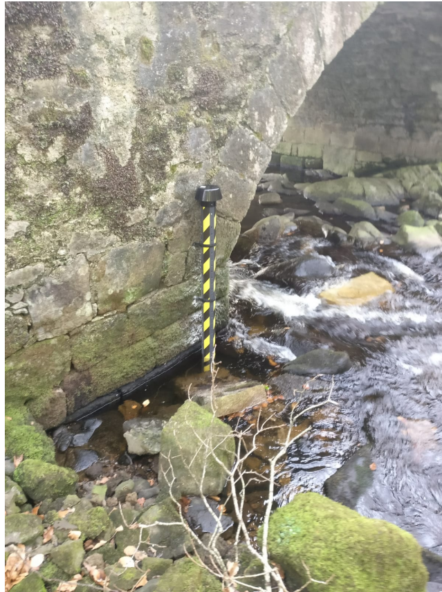
Figure 2.3: River level sensor that was used.
