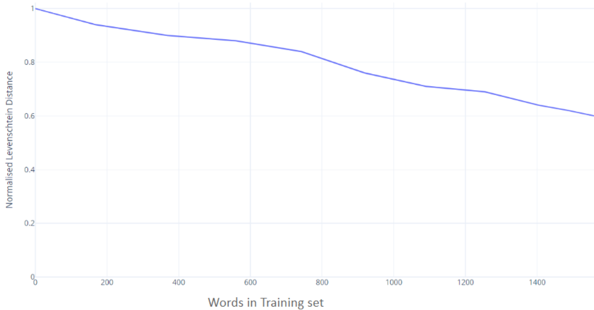
Figure 4.1: Comparison of the average normalised levenshtein distance against the amount of words used to train the neural network
