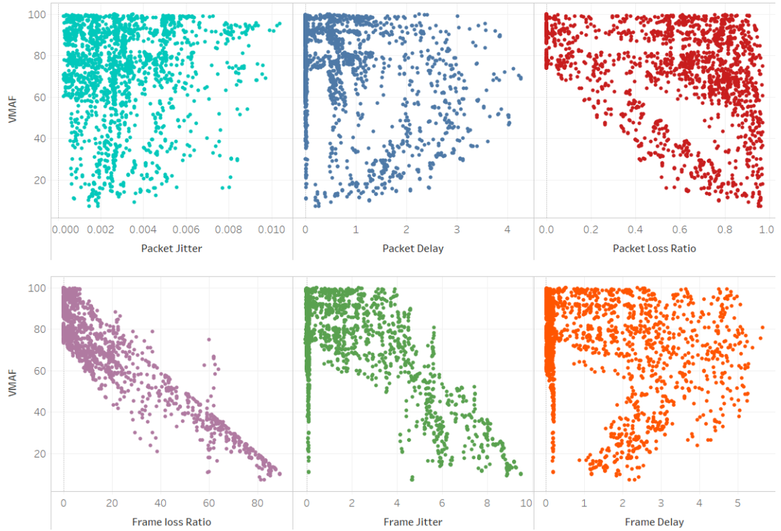
Figure 5.3: Scatter Plot of QoS Vs VMAF
