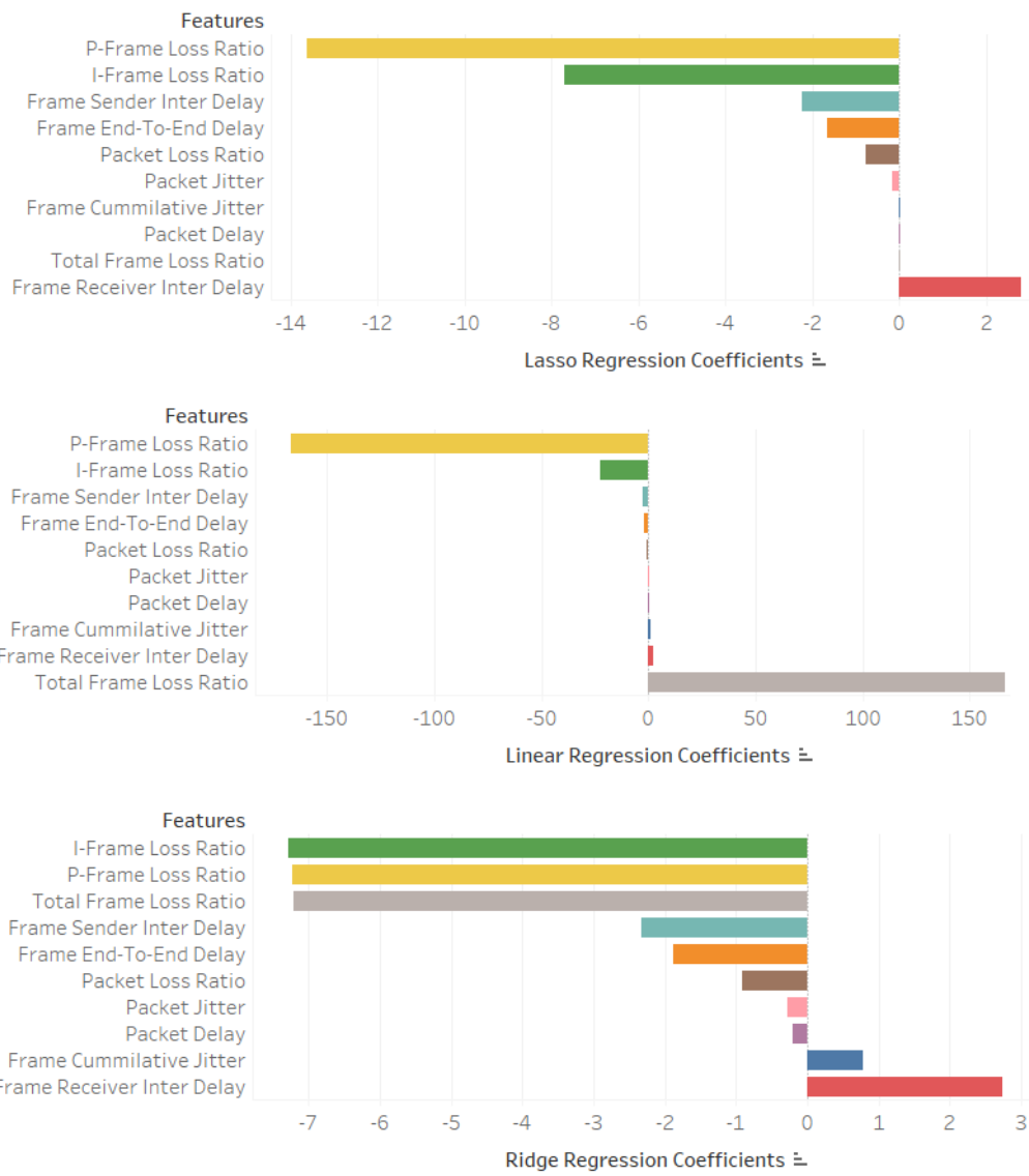
Figure 5.5: Coefficients of Linear models
