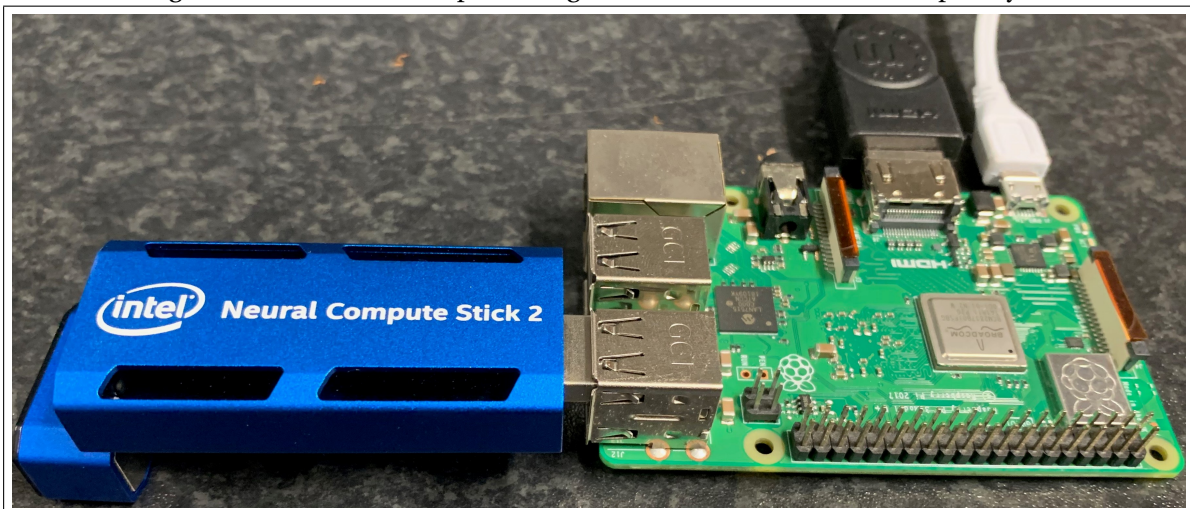
Figure 4.3: Hardware Setup showing Intel NCS attached to the Raspberry-Pi
