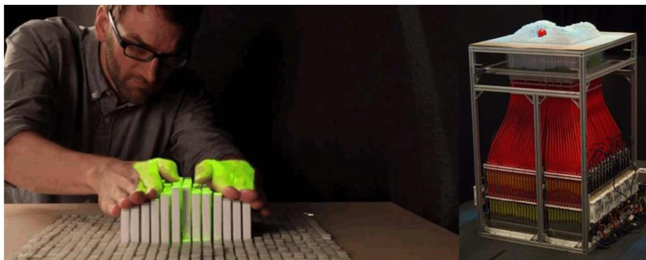
Figure 3 - MIT Media Lab InForm is a Dynamic Shape Display that can model 3D content physically, so users can interact with digital information in a tangible way (Bushel et al., 2018, p.105).
