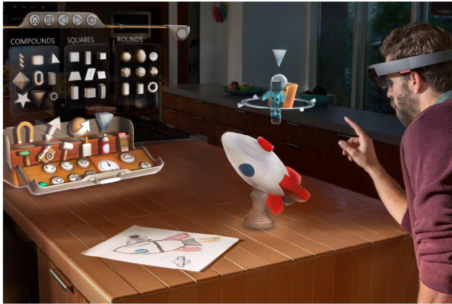
Figure 2 - Microsoft HoloLens is a consumer-level AR device that features instinctual interaction through gestures and voice recognition (Bushel et al., 2018, p.104).
