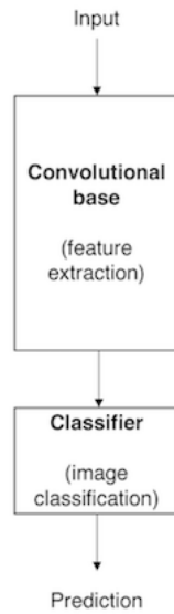
Figure 2.13: Simplified Architecture of CNN. Source:[8]
