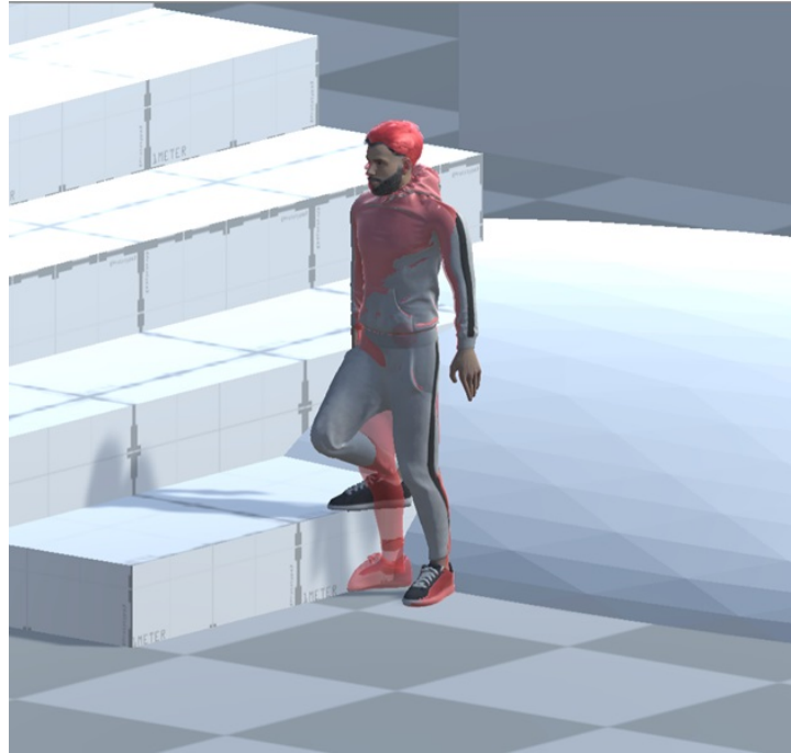
Figure 5.4: Leg adjustment using built-in IK system in Unity
