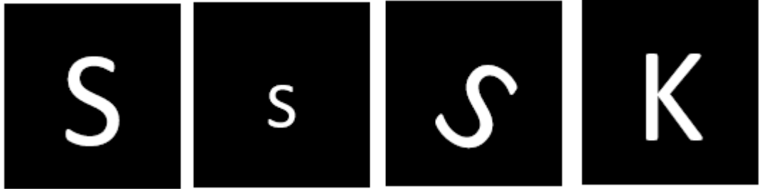
Figure 3.5: Letter S, having similar moment, in left 3 blocks showing change in image scale and rotation. Letter K, in right, will have different moment value.
