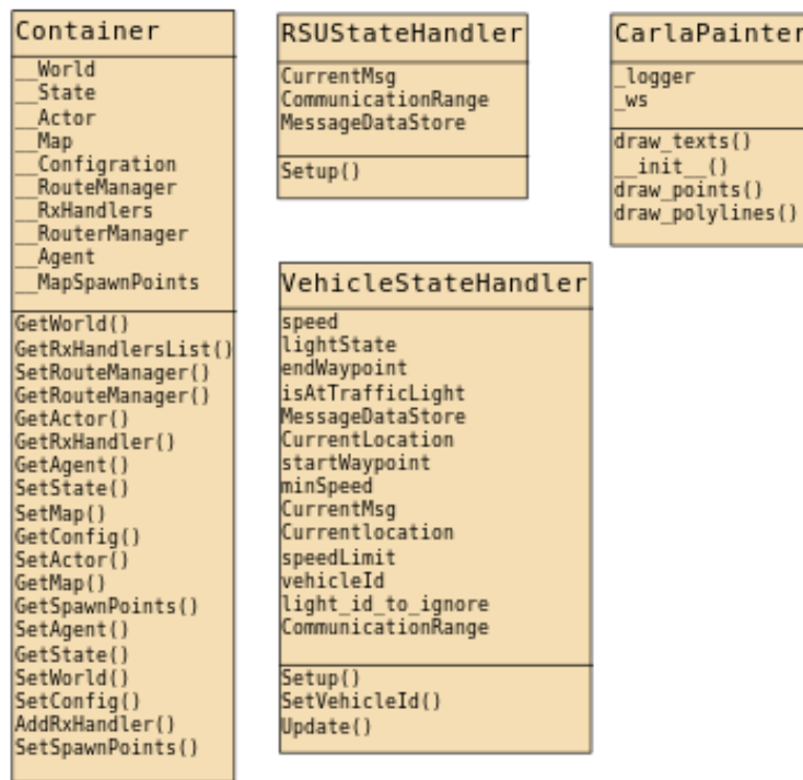
Figure 1: Class Diagram of Helper Component
