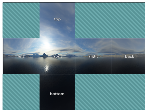
Figure 2.16: Cube-Map Projection visualised in rectangular image
