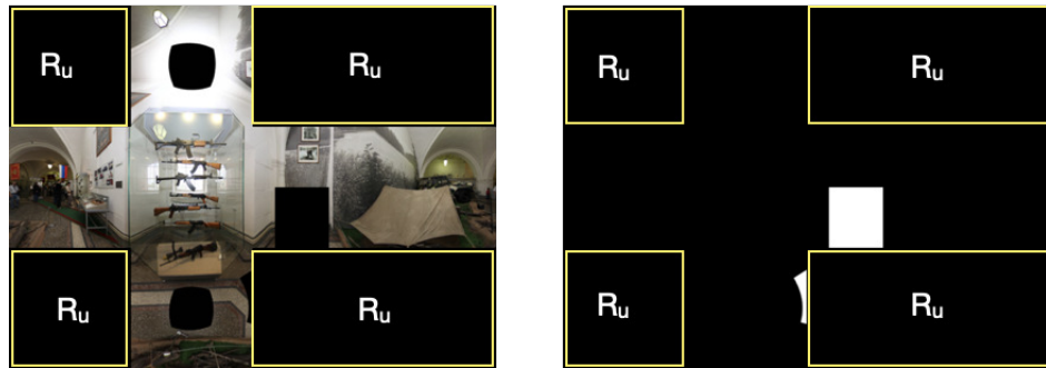
Figure 3.5: Cube Map input and mask conversion from Equirectangular projection
