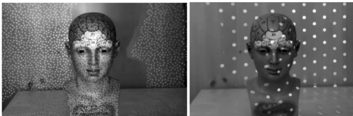
Figure 2.3: Obtained point cloud of front-facing face detection sensor on an iPad Pro 2020 on the left vs back-facing LiDAR sensor on the same device.
