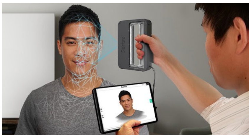
Figure 2.1: Example of passive non-contact scanning. Source: Sense 2 by 3D systems
