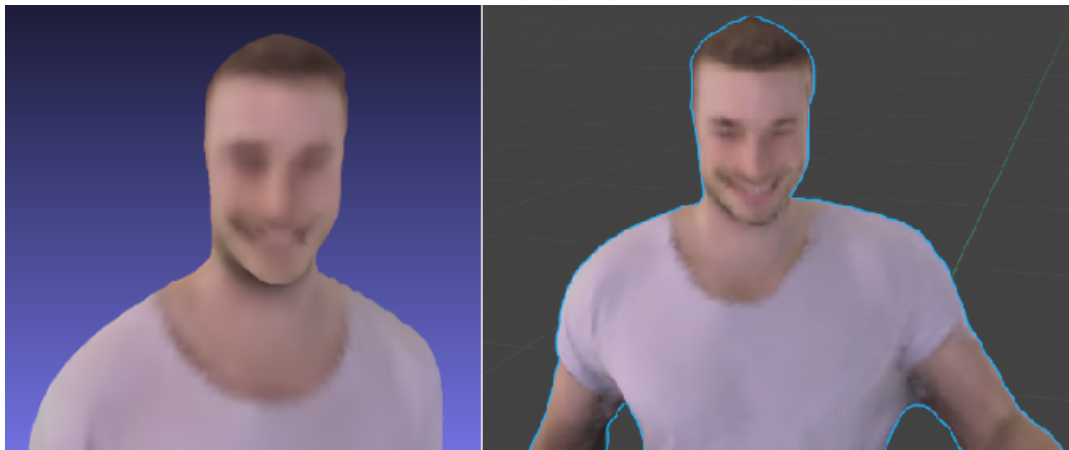
Figure 3.9: Visualization of the merged model without projection (left) and with projection (right)
