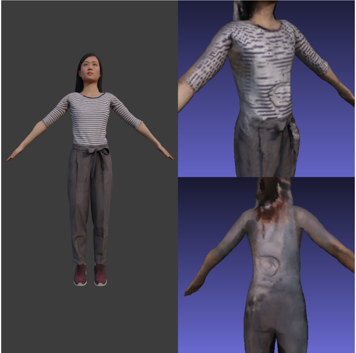
Figure 4.6: Another example of geometry artifact due to normal mapping, where the rest of the model remains unaffected. Input image (left), resulting model front face (upper-right) and resulting model back face (bottom-right)
