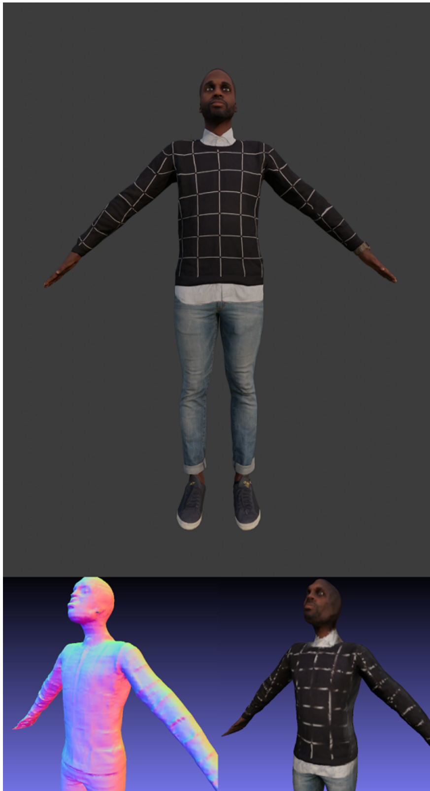
Figure 4.7: An example where a potentially glitch-causing clothes texture does not cause any disruptive geometry. Input texture (top), PI-FuHD generated model (bottom-left) and final model (bottom-right)
