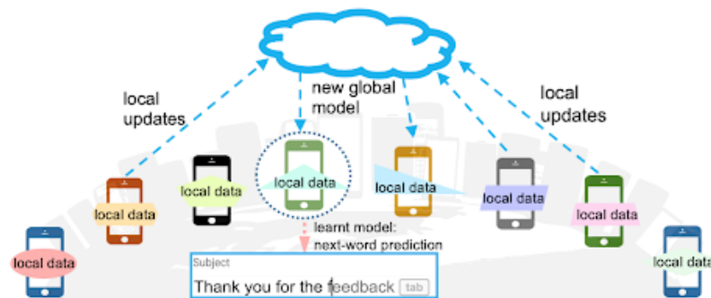
Figure 1.3: Figure shows in federated learning only the model updates are shared and the user data never leaves the edge device.
