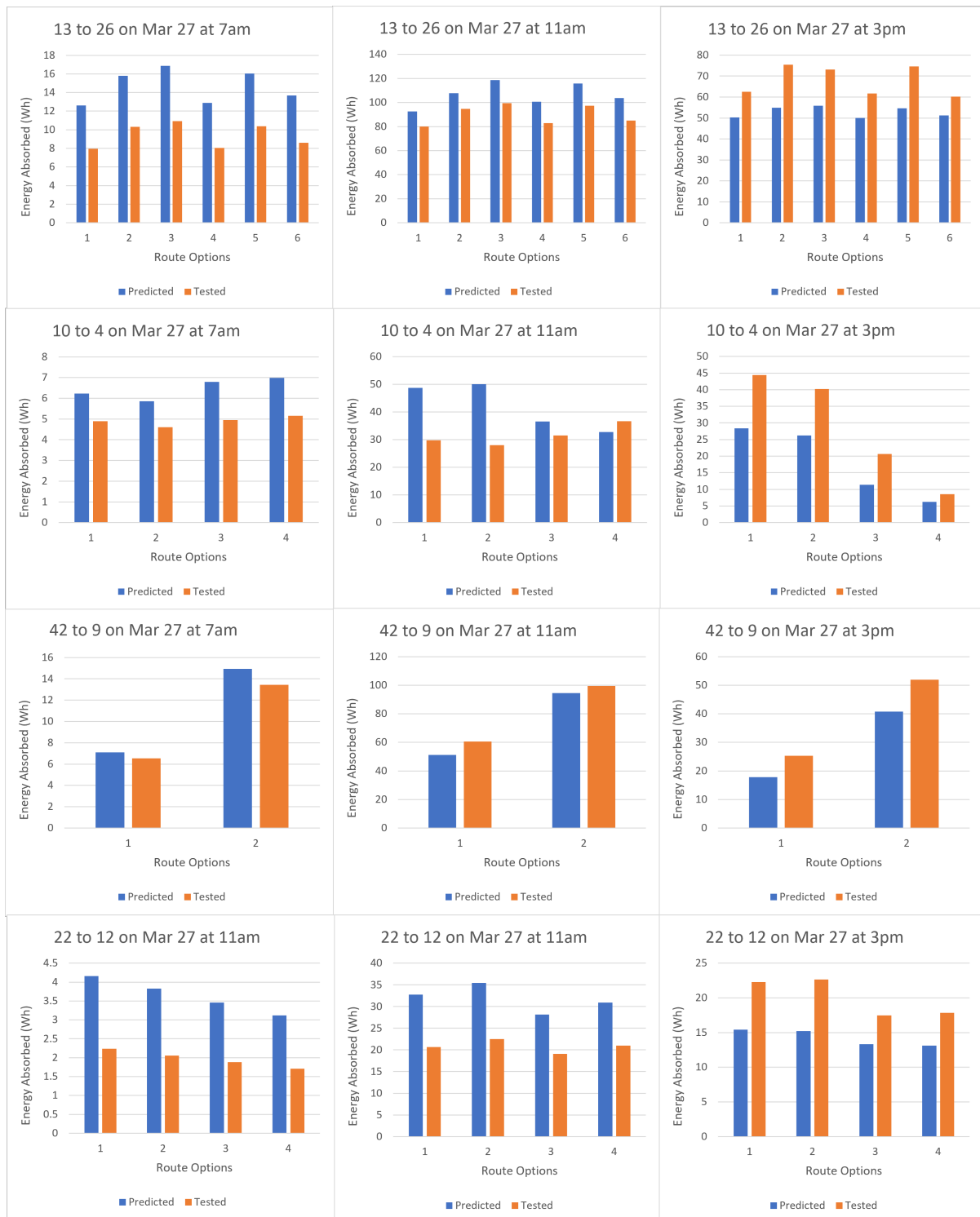
Figure 6.8: Comparison of predicted and tested data for solar absorption along a Journey
