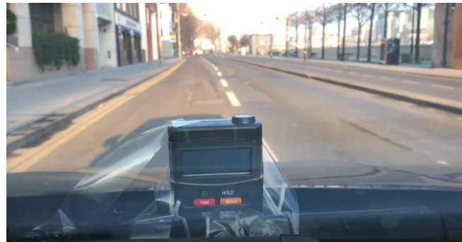
Figure 6.2: An image showing how the sensor was shaded by the car
