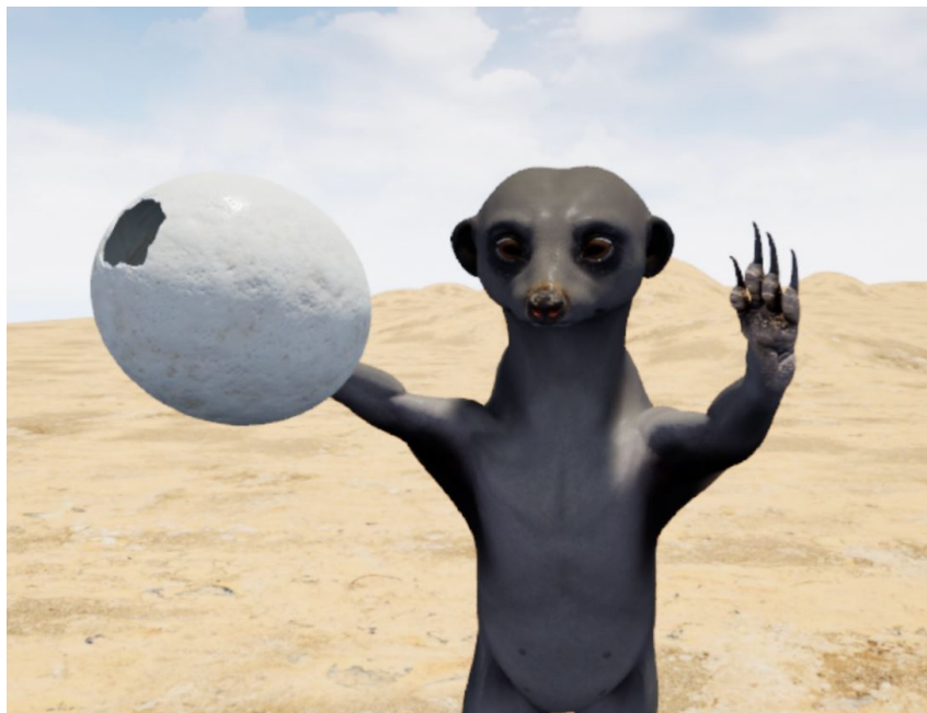
Figure 5.11: Image of the meerkat character grabbing an egg prop. The egg is added as a child of the "hand" bone to achieve this effect
