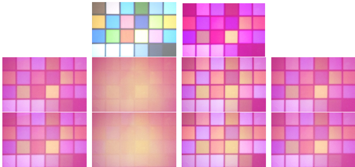
Figure 5.10: The image that projects the colour checker on the white background, and the images that project the baseline and all the results on the purple background. Extract the range we needed, and warp them into the same size. Images on the first line: target result and baseline. Image on the second line: (1):inverse RGB, (2):transfer RGB, (3):transfer RGB fix, (4):transfer RGB Inv. Image on the third line: (1):inverse HSV, (2):transfer HSV, (3):transfer HSV fix, (4):transfer HSV Inv
