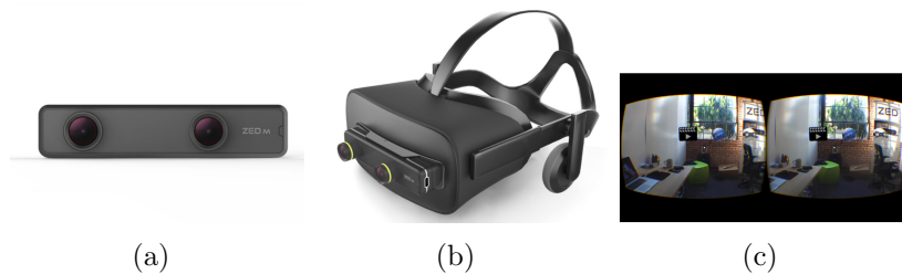
Figure 2.2: (a) Zed Mini Camera. (b) Zed Mini attached to the HMD. (c) the view returned by the Zed Mini.
