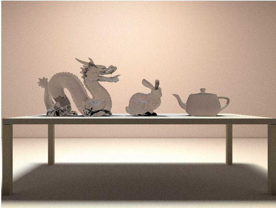
Figure 4: glass material model, SPP=500, bounce 8 times, cost 31minutes
