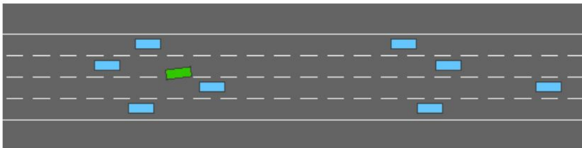
Figure 5.1: Screenshot of the fast-highway-v0 environment with CAVs (in green) and human-driven vehicles (in blue). In this figure the CAV is trying to change the lane to avoid collision with HDV.
