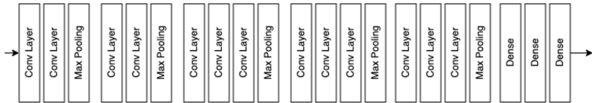
Figure 3.11: VGG16 Network Architecture
