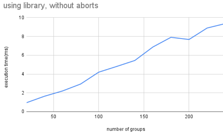
Figure 5.2: performance using the library with no retry for processes
