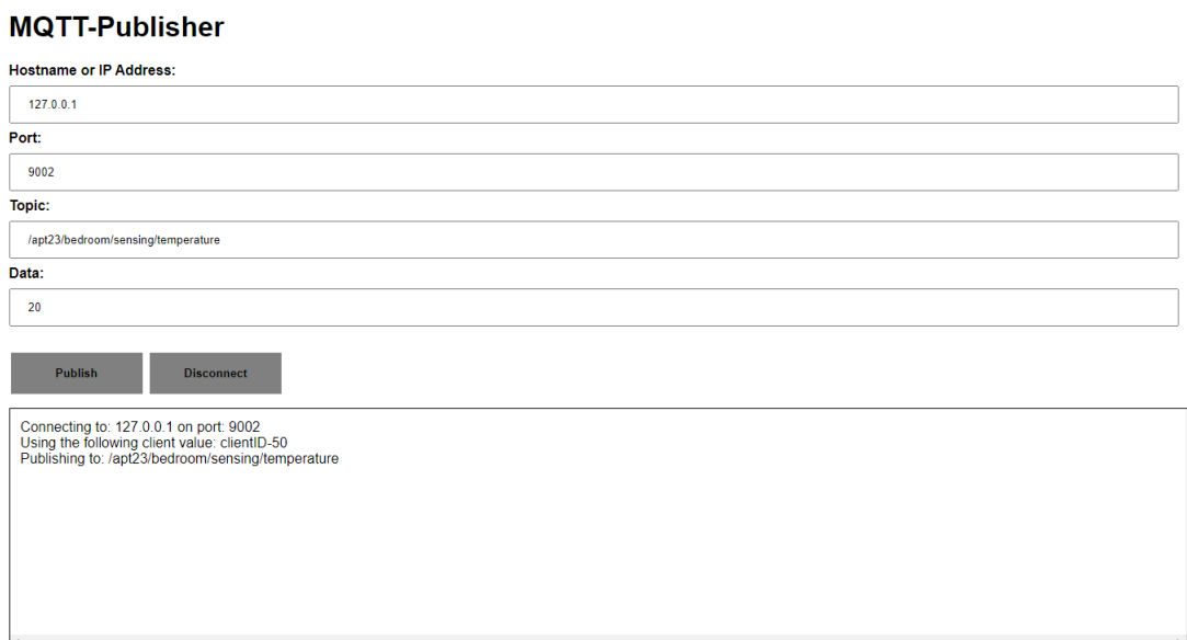
Figure 5.5: Webpage for MQTT client to publish data to broker1
