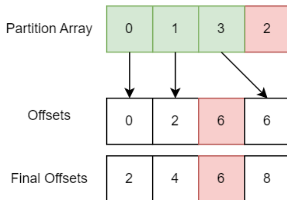
Figure 2.1: The Partition Array stores the indexes of unsorted partitions on the left-hand side of the array, marked in green, and sorted partition that no longer need to iterated over on the right-hand side.
