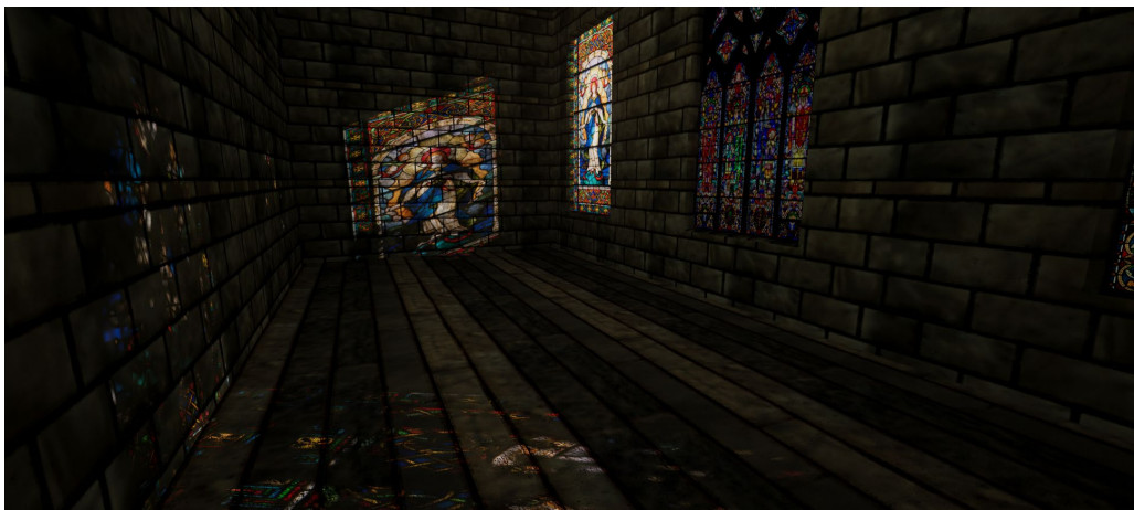
Figure 3.21: Attempting to apply one of the window images as a light cookie applies it repeatedly to all light cast by the sun, leading to uncanny and unrealistic results
