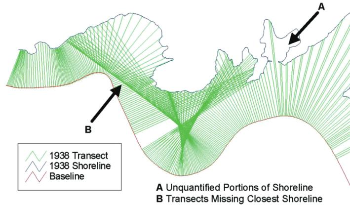
Figure 2.5: An example visualisation of two problems present with the transect from baseline method for measuring coastal change. Area A of the coastline shows portions of the coastline not represented in this methods analysis. Area B shows how the nearest coastline areas can be missed, and as such will overlap with other transect lines. This figure originated from Smith and Cromley (2012).
