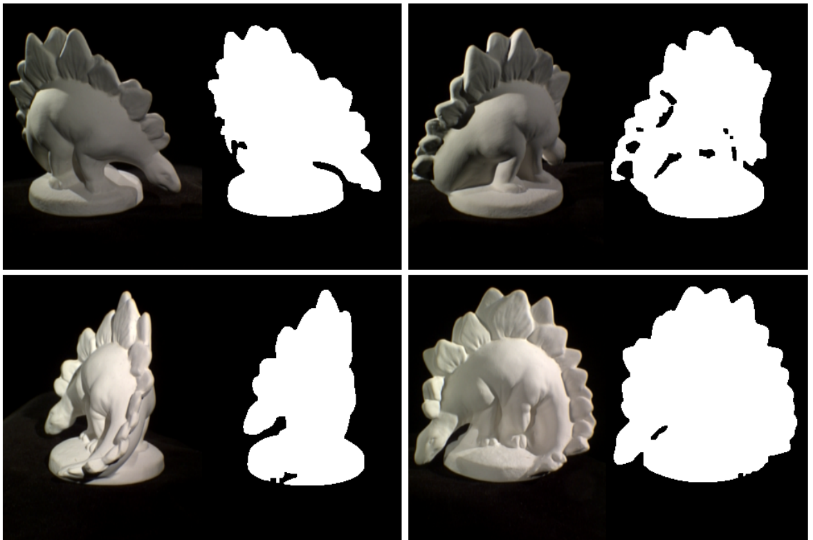
Figure A.5: Left images illustrate captured images from different views in the Middlebury database (67), and its silhouettes segmented by a background subtraction method are shown in the right. The silhouettes are not perfect due to shadows on the dinosaur.
