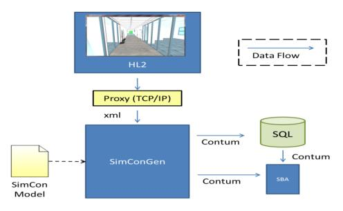
Figure 5-12 Data Communication between the VR Building, the SimCon Generator and the SBA.
