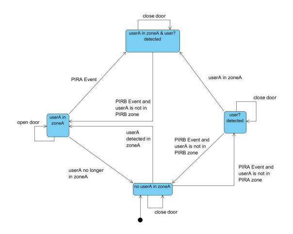
Figure 6-21 Automatic Door Finite State Machine
