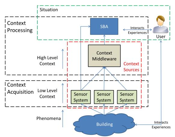
Figure 2-1 Context Acquisition and Processing, resulting in low and high level context and ending in a situation
