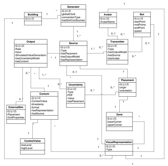
Figure 4-4 UML Class Diagram: SimCon Model
