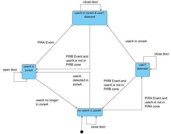
Figure 16-3 Automatic Door Finite State Machine
