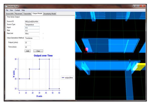
Figure 5-9 Output Model: Temperature SimCon Source Modelled as Time Series
