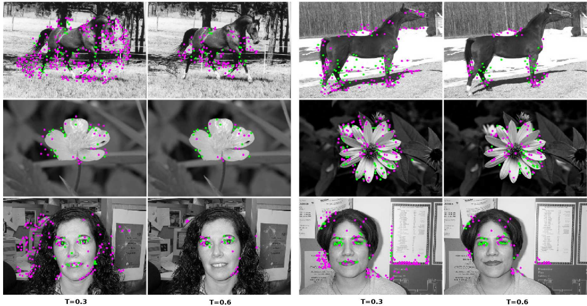
Figure 3.3: Example results for \mathbf{T} = 0.3 and 0.6 . From top to bottom: horses, flowers and faces. Green dots indicate feature points classified in the image class ( \mathbf{C} ), purple dots indicate feature points classified outside of it ( \bar{\mathbf{C}} ).
