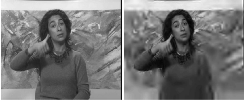
Figure 1.1: Foveated imaging example of a woman doing sign language. Image on right has its resolution adapted around the woman’s hand and face (taken from [175]).
