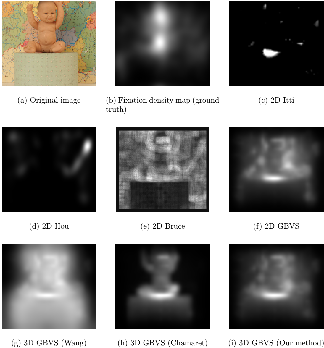
Figure 4.3: Saliency maps with VSAs. (a) Original image #2 [173], (b) Corresponding fixation density map, (c)-(f) Saliency predictions from the four 2D VSAs: Itti, Hou, Bruce and GBVS, (g)-(i) Saliency predictions from the three 3D VSAs: 3D GBVS (Wang), 3D GBVS (Chamaret) and 3D GBVS (Our method)
